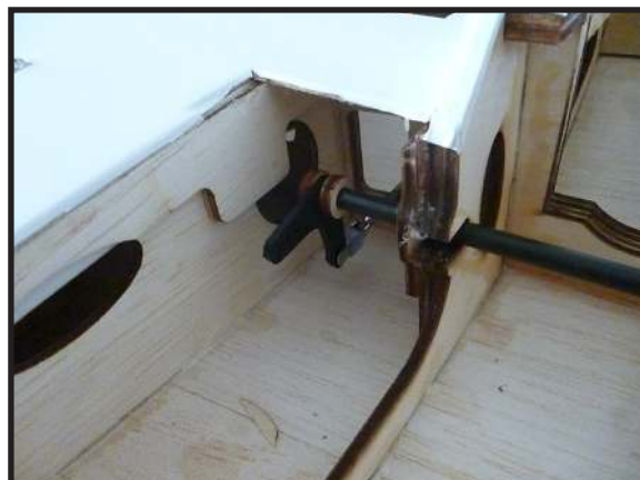
Finished gear door servo/control rod.
