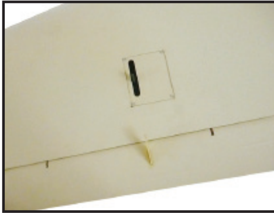
INSTALLING THE FLAP SERVOS.
