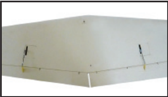
INSTALLING THE RUDDER SERVO.
