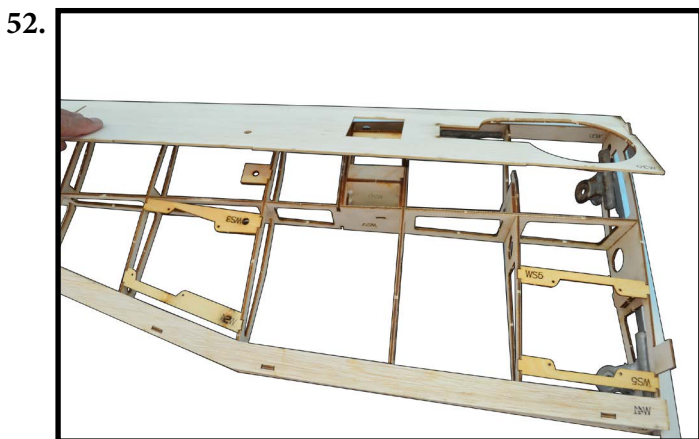
- Cover the balsa sheet W39 with balsa frame W25 available to wing .
