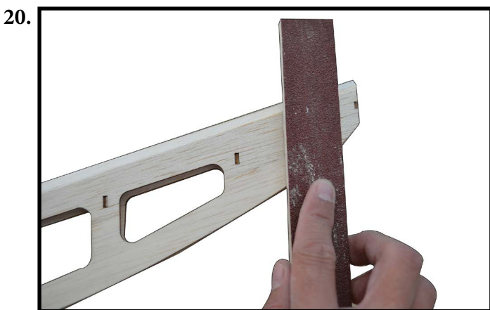
- Use sandpaper bar for sanding leading edge WA20.
