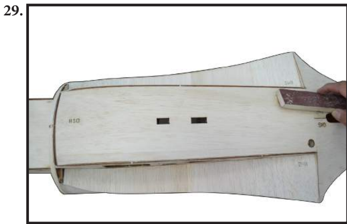
- Fitting the hatch into the fuselage, and then use the Sandpaper Bar to sanding at the area contact with the fuselage, on forward , also on behind so that setting up the hatch and the fuselage fit together.
