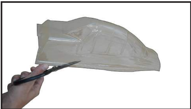
- Cut off redundant cy plastic around.
