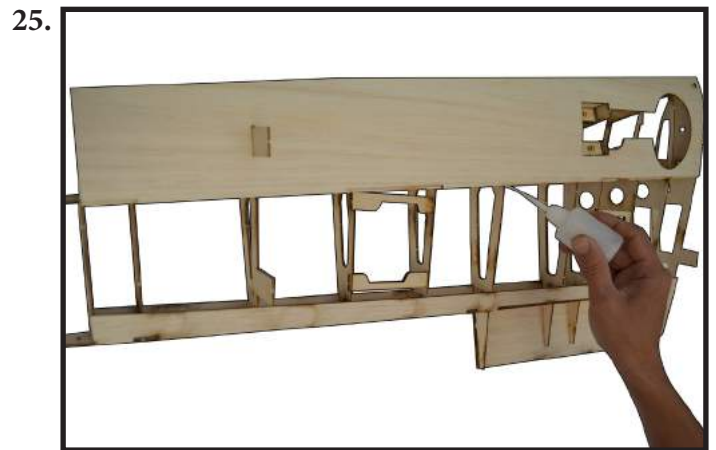
- Cover sheeting W38 and then add more CA Glue.
