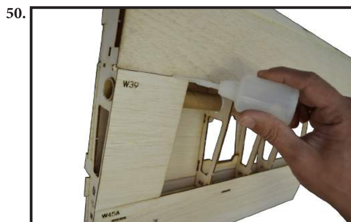
- Paste the sheet W39 on the ribs and add more CA Glue.
